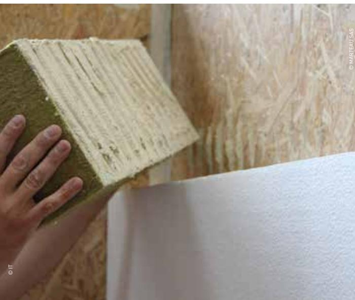
▲ LA LAINE DE ROCHE EST ISSUE DE LA FUSION DU BASALTE (PIERRE NOIRE D'ORIGINE VOLCANIQUE) OU DE LAITIER DE HAUTS FOURNEAUX (PRODUIT CRÉÉ LORS DE LA FABRICATION DE LA FONTE) ET DISPOSE D'UNE EXCELLENTE RÉSISTANCE AU FEU.
